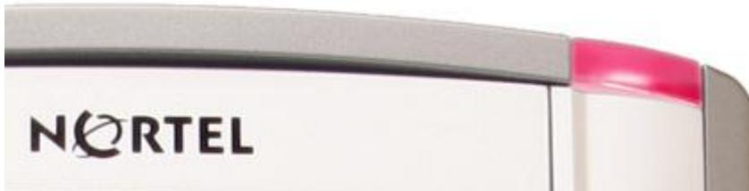
When a message is waiting, the Red **Visual Alerter/Message Waiting indicator** flashes. Also, this indicator flashes when the telephone ringer is on.
